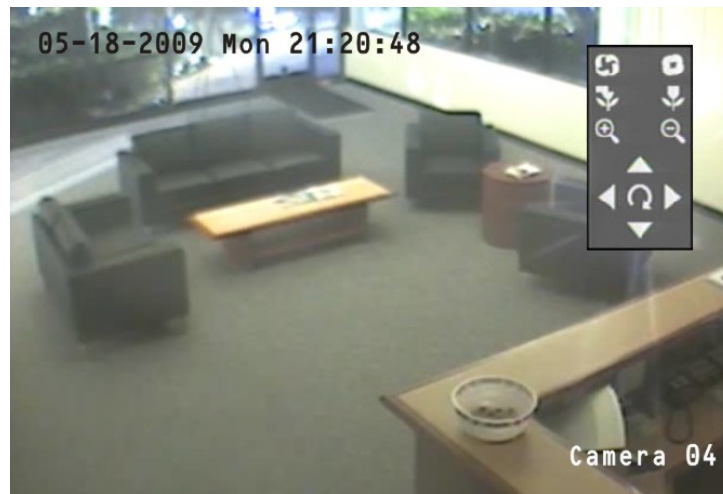
Figure 12: PTZ control interface
